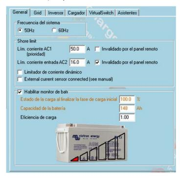
Select the Charge current in function of the number of batteries. 25<sup>a</sup> \* No of modules
