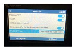
2. SYSTEM SETTING → TURBO ENERGY battery on CAN-BUS
